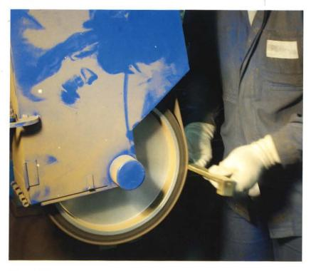
**Above:** Polishing a piece of raw brass. This operation removes any scratches by "wearing down" the piece, rubbed against a series of buffers or pads to obtain a smooth and uniform surface appearance.
