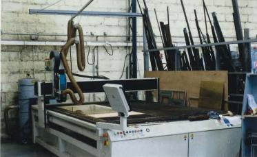
**Top:** The VLD workshops, in Ivry-sur-Seine, cover an area of over 800 m<sup>2</sup>. **Bottom:** This 3-D digital drilling machine is used for engraving motifs, cutting out templates and manufacturing railings.
